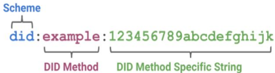
Figure 8.x: The general format of a DID—the scheme name followed by a DID method name followed by the method-specific string, the syntax for which is defined by the DID method
