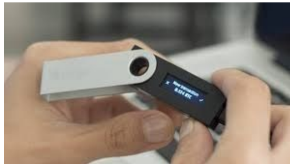
Figure 2.7: A typical dedicated hardware wallet for cryptocurrencies. This one is called Ledger Nano S and has its own secure display.
